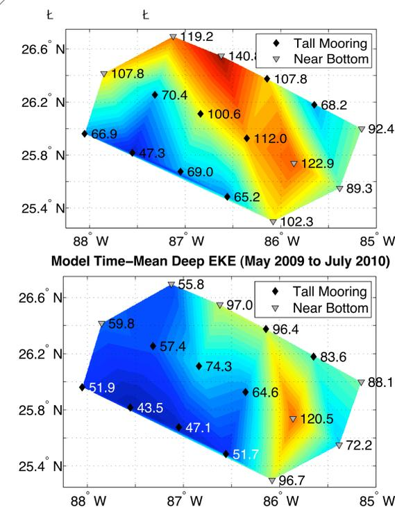
Similar patterns of time-averaged deep EKE were observed in the model and array. Units are  $\text{cm}^2 \text{s}^{-2}$ .
