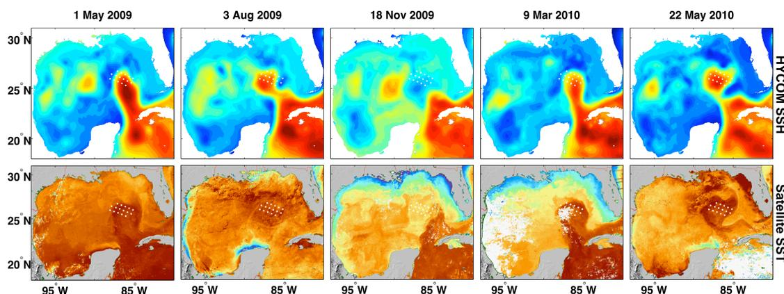
In the 15 months of data acquisition (Apr. 2009 – Jul. 2010), two LC eddies formed and separated. The August 3<sup>rd</sup> and May 22<sup>nd</sup> panels show the formation of LCEs Ekman and Franklin respectively. Mooring locations indicated by white dots.
