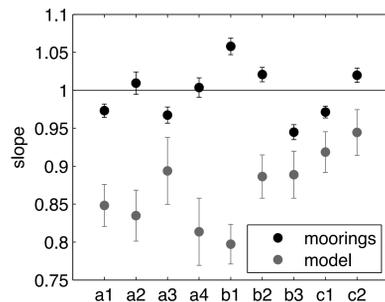
A comparison of bottom trapping between array tall moorings (black) and GOM HYCOM modeled tall moorings (gray) shows greater trapping in the model.
