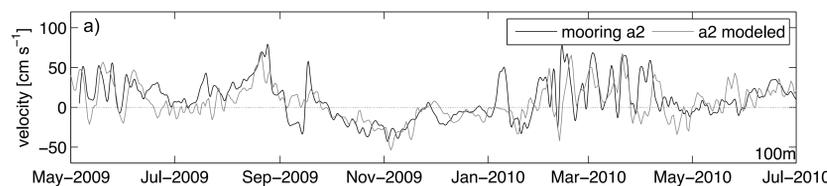
A time-series comparison between mooring a2 (black) and modeled (gray) velocity at 100 m shows coinciding peaks of high/low velocity. Bunched peaks correspond to eddy separation events.
