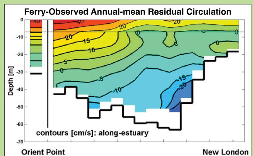
Surface current in southern portion of crossing (nearer Orient Point) LEAVES Long Island Sound at fastest rate. Bottom current in northern portion of crossing (nearer New London) ENTERS Long Island Sound from the ocean at fastest rate.
