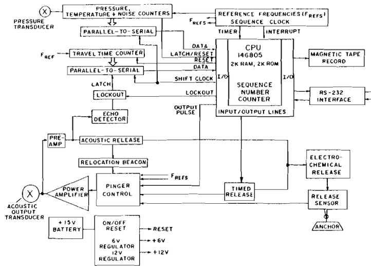
Fig. 1 BLOCK DIAGRAM OF INVERTED ECHO SOUNDER
