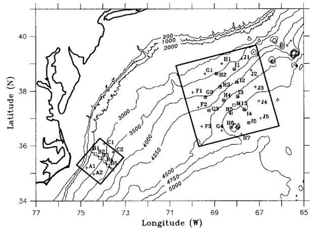
FIG. 1. The SYNOP Inlet and Central Arrays. Inverted echo sounder sites are denoted by the plus symbols and current meter moorings by the open squares. The bold boxes indicate the regions that have been mapped by optimal interpolation. Bathymetric contours are in meters.
