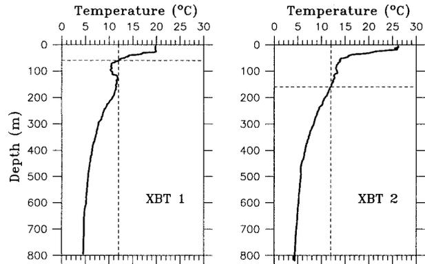
FIG. 3. Temperature profiles of two XBTs used to calibrate an IES. The dashed lines highlight the 12°C isotherm depth.
