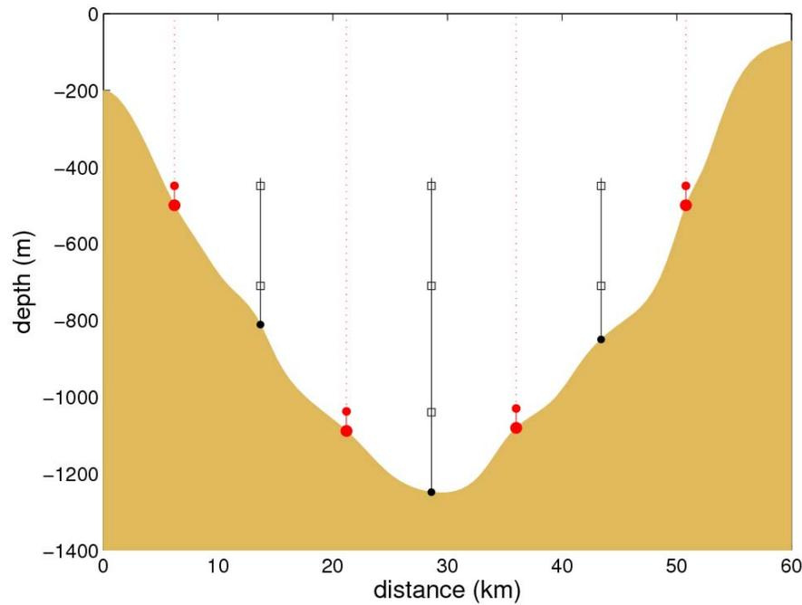
*Figure 2. Proposed Kerama Gap array. Four CPIESs are shown as solid red dots (smaller upper dot represents the position of the current sensor 50 m above the sea floor). Seven CMs on three moorings are shown as open squares. Note: this section across the Kerama Gap is slightly northwest of the sill, hence the maximum depth at the section is greater than the sill depth (1050 m).*
