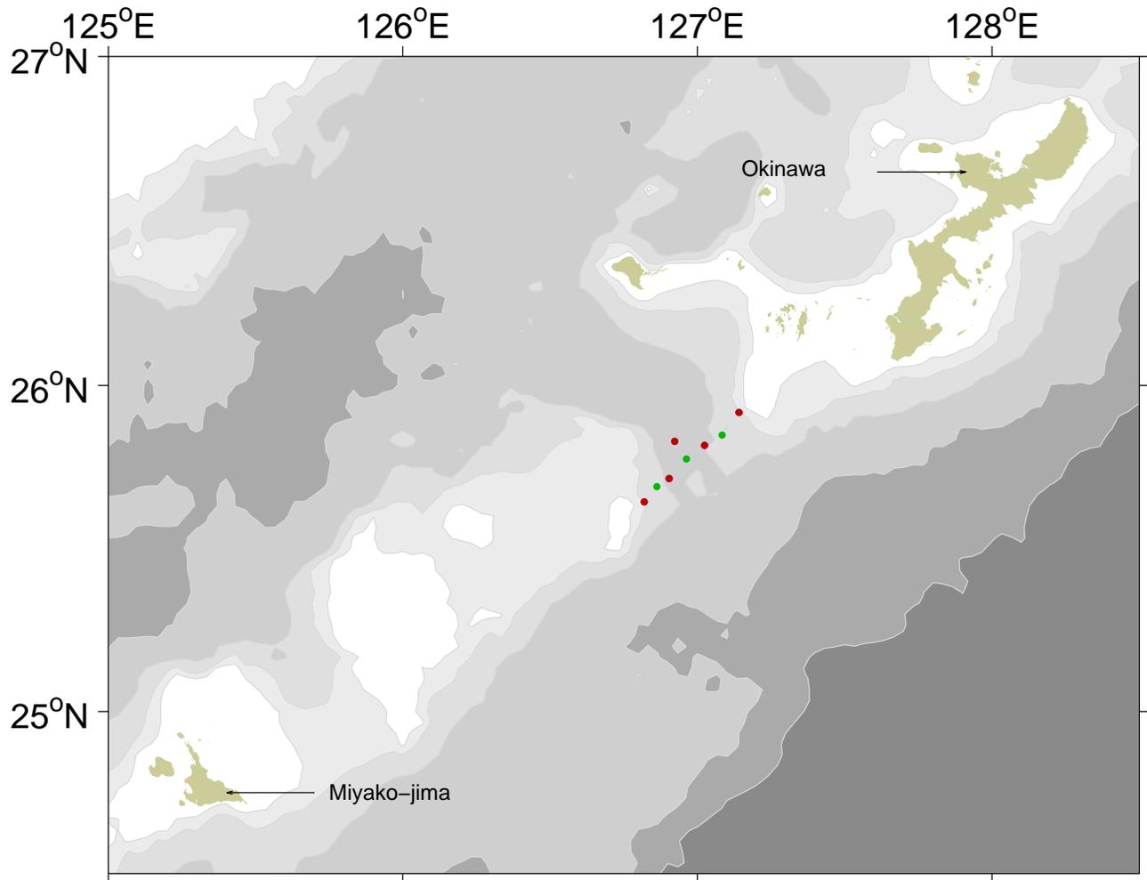
**Figure 3.** *The Kerama Gap array, as deployed in June 2009, consists of five CPIES instruments (red dots) and three current-meter moorings (green dots). The array is along a line across the Kerama Gap, except that one CPIES instrument near the center of the Gap is about 10 km northwest of this line. Depth contours are at 200, 500, 1000, 2000 and 3000 m.*
