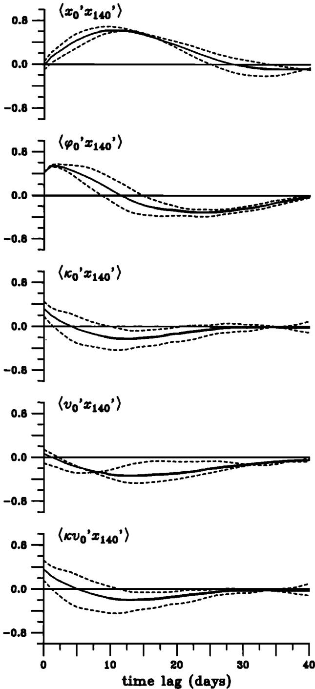
Fig. 5a. Cross correlations between the detrended Inlet parameters (Inlet displacement, angle, curvature, velocity, and curvature vorticity) and the time-lagged detrended displacement at 140 km from the Inlet. The solid lines are the cross correlations computed from the entire 740 days. The two dashed lines in each plot are the cross correlations computed from the first year and from the second year.
