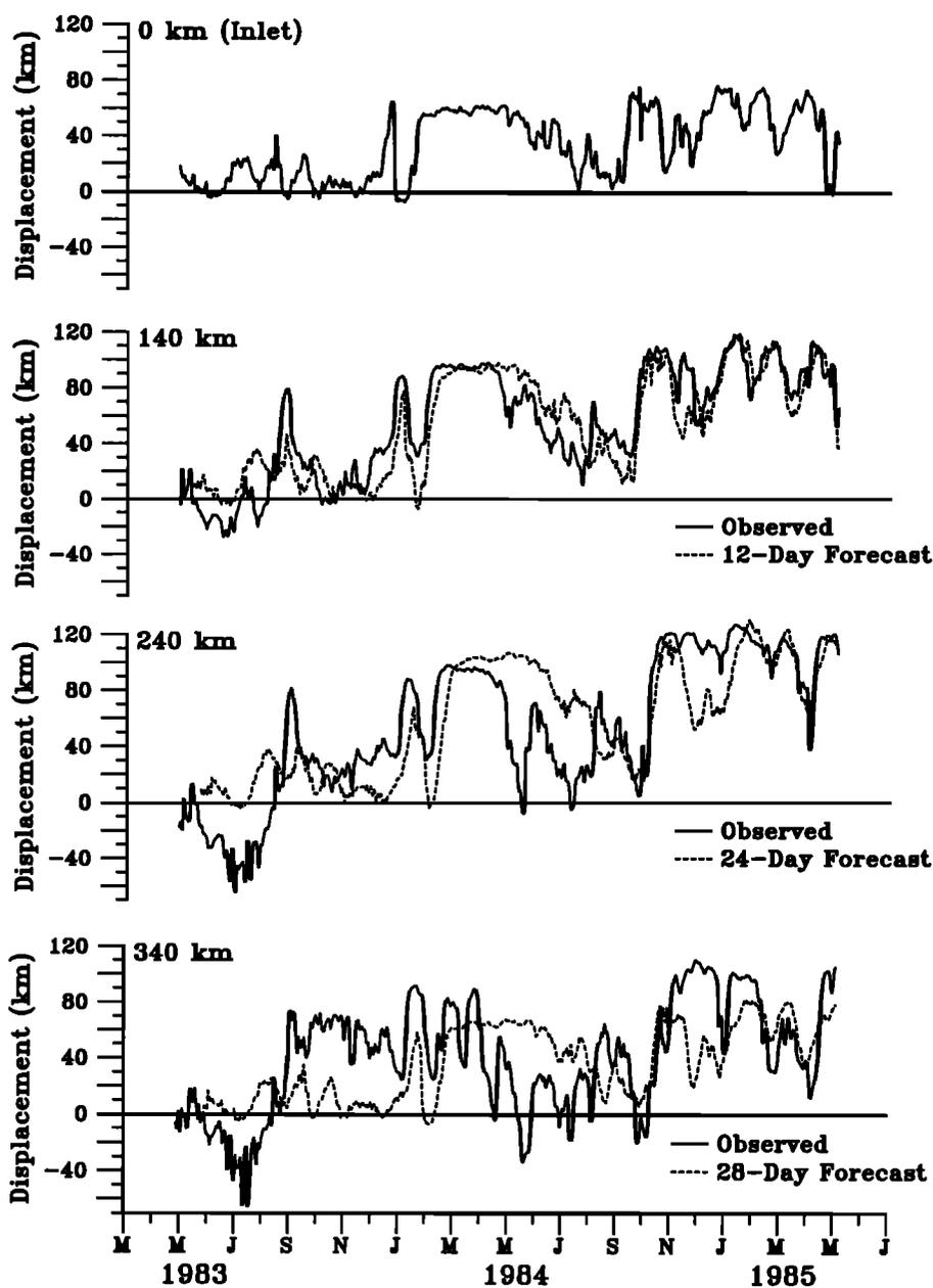
Fig. 3. The measured displacements (solid lines) and first scheme's forecasted displacements (dashed lines) at 140 km, 240 km, and 340 km from the Inlet. The measured Inlet displacement, which was used as a predictor, is shown in the top plot.
