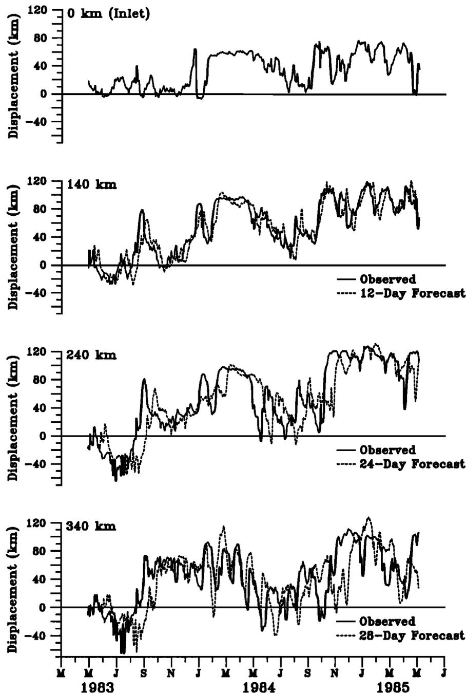
Fig. 6. The measured displacements (solid lines) and second scheme's forecasted displacements (dashed lines) at 140 km, 240 km, and 340 km from the Inlet. The measured Inlet displacement, which was used as a predictor, is shown in the top plot.
