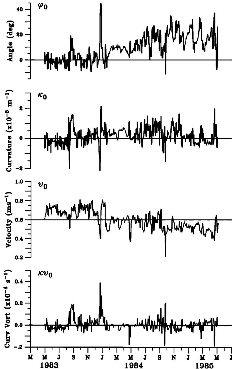
Fig. 2a. Inlet parameter time series (angle, curvature, velocity, and curvature vorticity), measured by the inverted echo sounder array.
