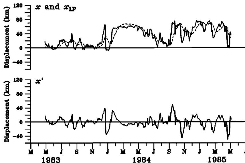
Fig. 4. The Inlet position time series (upper plot, solid line) decomposed into a trend (upper plot, dashed line) and a perturbation time series (lower plot) using a causal, second-order, 150-day high-pass Butterworth filter.
