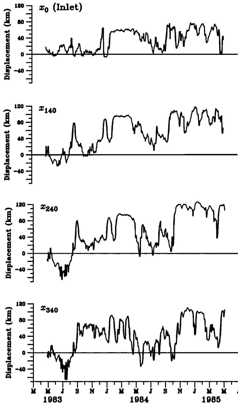
Fig. 2b. The displacement time series at the Inlet, and 140 km, 240 km, and 340 km from the Inlet, measured by the inverted echo sounder array.
