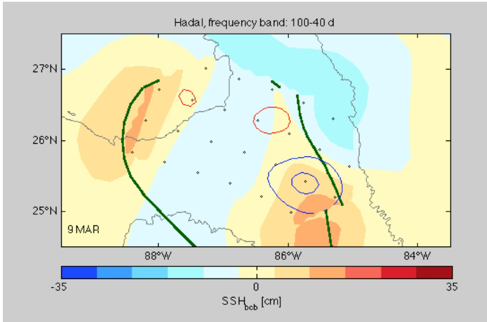
Upper Loop Current--- filled contours    Deep eddy field --- lines
