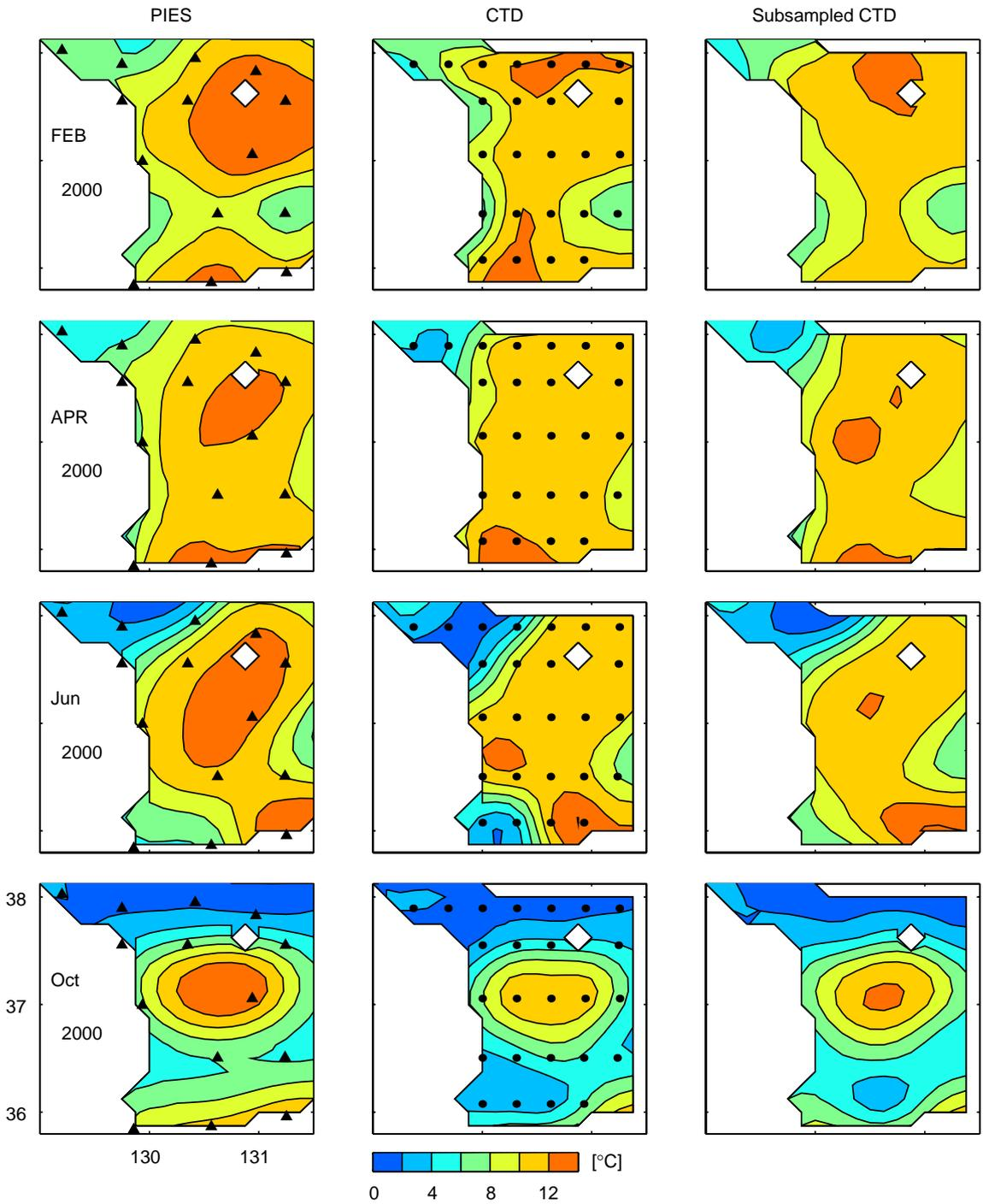
Fig. 9. Optimally interpolated maps of temperature at 100 dbar generated from PIES data interpreted with the Residual GEM Technique (left column) and generated from Korean CTD data (center column) in February, April, June, and October 2000. The PIES data were averaged over the duration of the CTD collection period. Contour interval is 2 °C. PIES locations are marked by black triangles and CTD locations by black dots. Right column: CTD data subsampled to PIES locations.
